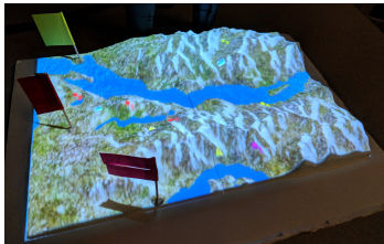
Figure 2: A prototype of a tangible interface for supporting SAR managers in building and maintaining a bigger-picture awareness of a search response.
