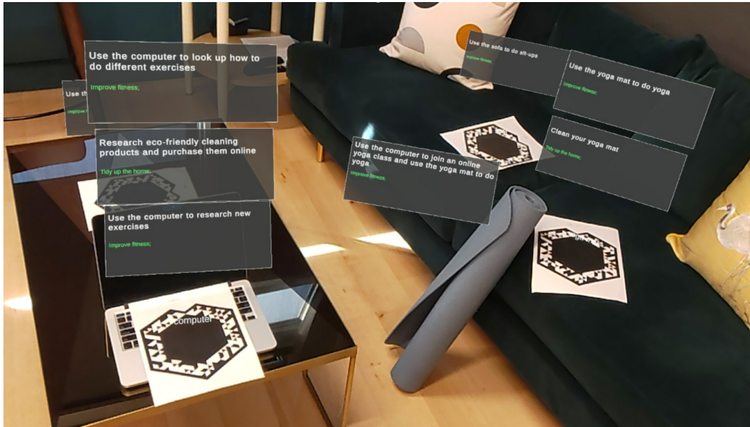
Fig. 1. The AR prototype displaying situated action recommendations next to relevant objects in a mock apartment space.
