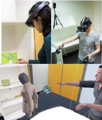
Figure 4: In Mini-Me [13], remote (VR) user (up, right) enters a 3D modeled world (bottom) that maps to the real space of the local (AR) user (up, left).
