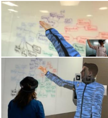
Figure 7: In the VROOM system [8], the remote (VR) user has a 360° camera view of the local space, as well as ability to use hand gestures (top). Bottom image shows the remote user's avatar in the local (AR) user's view.
