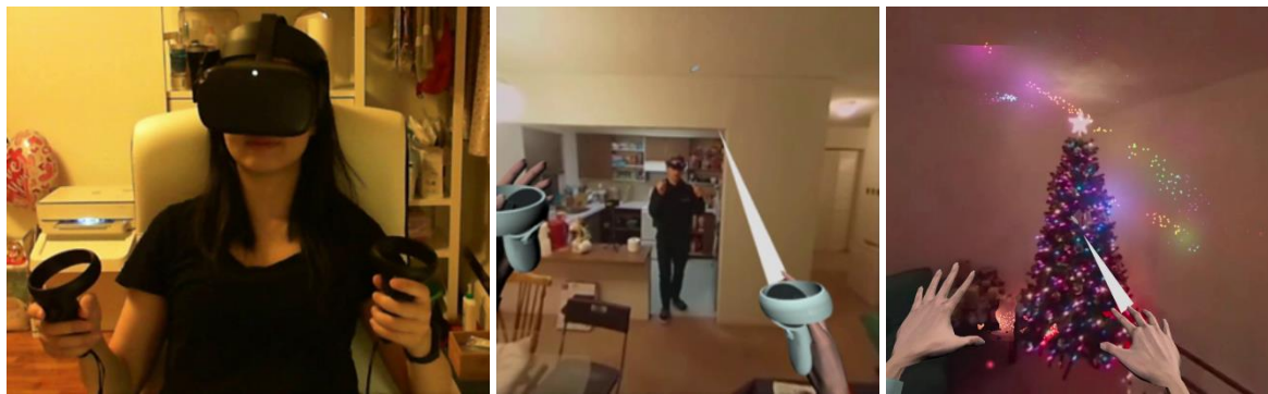
Figure 2: The XRmas telepresence system, VR side. The left photo shows the remote user wearing a VR headset in their environment. The centre and right photos show the remote user's view (through an Oculus Quest VR headset) into the local user's environment.
