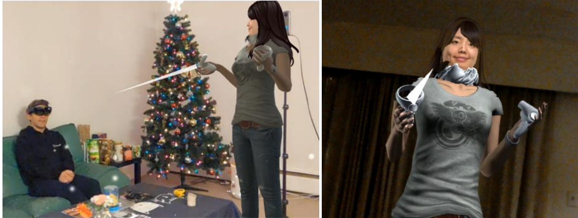
Figure 1: The XRmas telepresence system, AR view in the local environment. The left photo shows the local user sitting on the sofa and interacting with the remote user's avatar. The right photo shows the local user's first-person view (through a Microsoft HoloLens AR headset) of the remote user's avatar.
