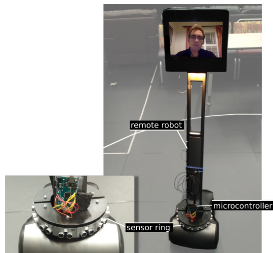
Figure 2: The ring consisting of 12 ultrasonic distance sensors attached to the Beam+ telepresence robot enables 360° coverage with a radius of up to 4m.
