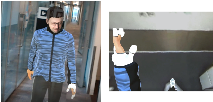
Fig. 3. Left: The remote user's avatar overlaid on the robot, as it appears in the local user's HoloLens. Right: The remote (VR) user's 1st-person view of their own avatar, looking down at their avatar's body.
