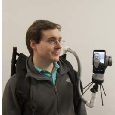
Figure 2.3: A camera, worn on the local user’s shoulder, that can be mechanically controlled by the remote user. Source: Kratz et al. [32]
