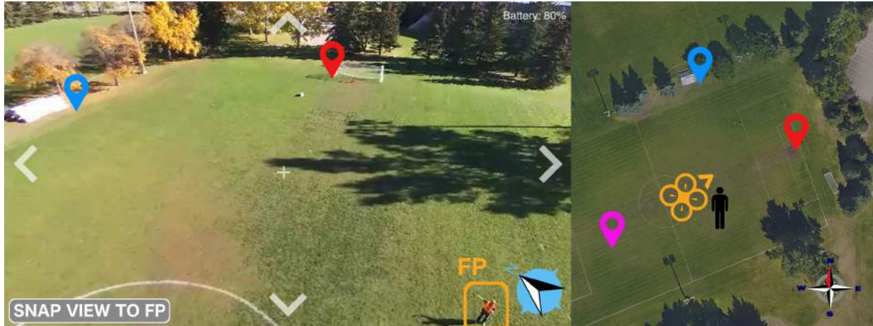
Figure 5.2: An interface mockup illustrating some potential features that could address the challenges of establishing orientation and finding objects in the activity space. The features shown in the mockup are: an annotation highlighting the FP’s location in the drone view, a button for snapping the drone view to show the FP, a map showing the locations and orientations of the drone and the FP, a compass indicator in the drone view indicating the orientation of the camera, and world-stabilized pins on the map and in the drone view indicating certain objects and points of interest.
