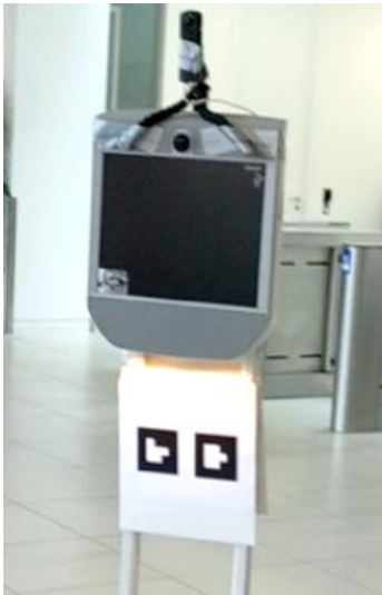
Figure 8: An earlier version of the robot setup with the marker pattern (bottom) and 360° camera (top).
